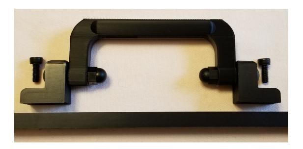
4. Attach the bottom bracket to the radio using 4 M4 x 10mm stainless button head screws. The front of the bracket is jogged a bit to accommodate the bezel of the radio, it only fits one way. You should be able to tighten these screws firmly, but do not use excessive force.
