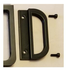
2. Assemble the handle and the two handle brackets using the 2 M5 x 25mm socket head screws, and the nylon cap nuts. The screws go through the thicker part of the bracket. They are a tight fit, so you may need to twist the screw through the bracket to get it to go all the way. Tighten the cap nuts firmly - it may appear that the handle motion is stiff, but this will loosen a bit with use.
